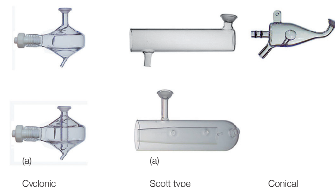
Fig. 2 Common spray chamber types; a: double pass designs
