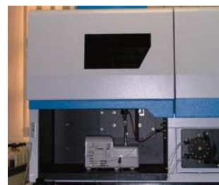
Image 1: cooled cyclonic spray chamber (Peltier effect), below the torch compartment.
