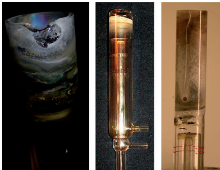
Figure 5. Common wear from high temperature and presence of high TDS.
